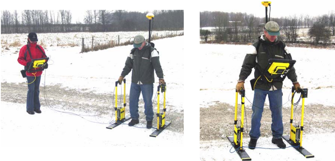
Figure 6-9: Two person (left) and one person (right) system configurations with GPS added. Ideally, the GPS should be positioned near the mid-point of the GPR antennas.
