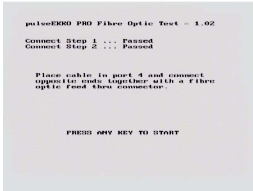
Figure 7-6: After connecting the fibre optic cable as shown in Figure 7-5, select System Setup - Acquisition Control - Fibre Optic Testing.
