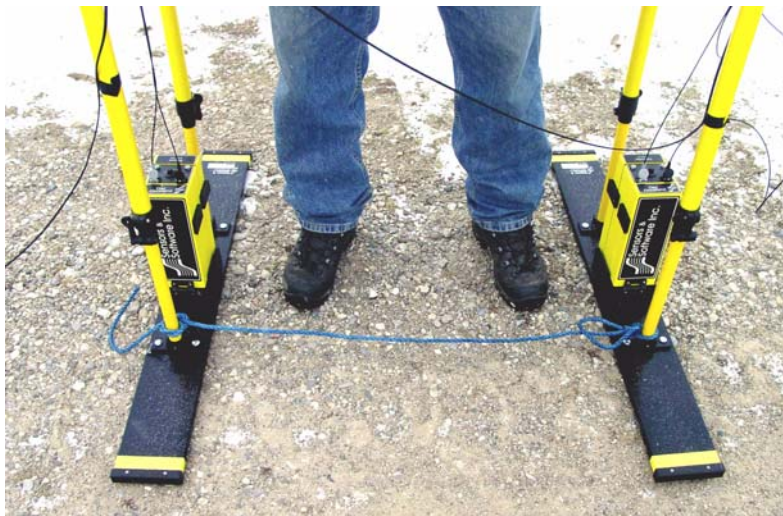
Figure 6-4: When using the adjustable handles, the antenna separation can be maintained by using a length of rope tied between the antennas.
