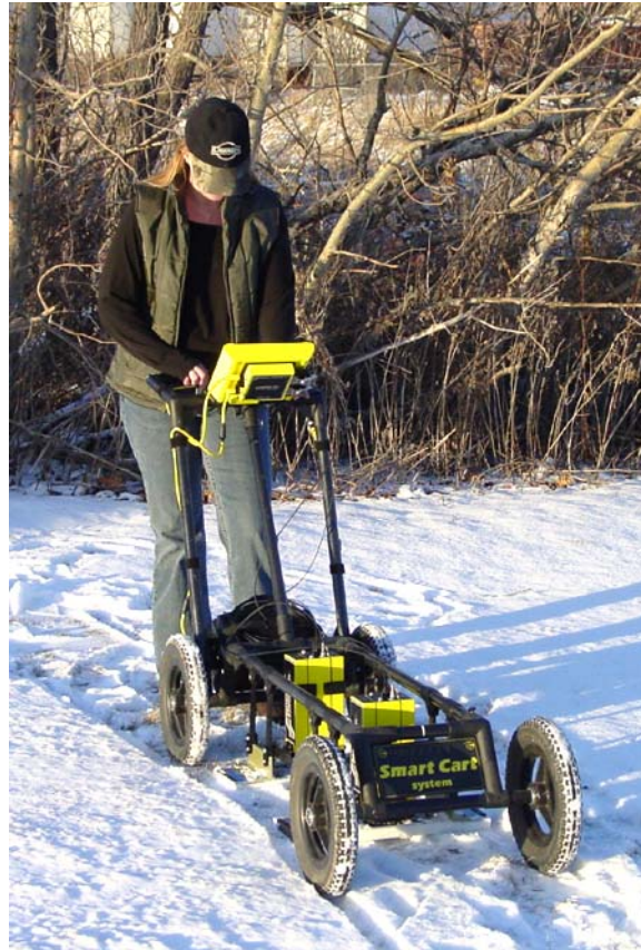
Figure 6-8: The pulseEKKO PRO SmartCart has an odometer to trigger the system to collect data at an equal step size defined by the user.
