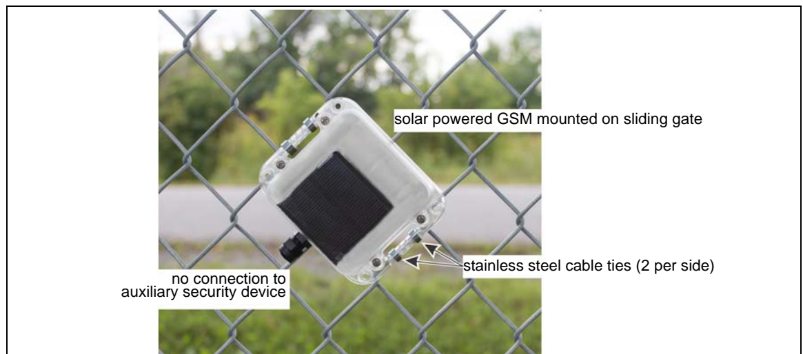
Figure 1 FlexZone Wireless Gate Sensor Module (solar powered)
