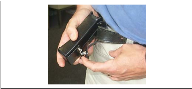
Figure 2: Opening the security snaps
