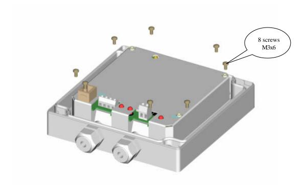
Step 6 – Internal Antenna Assembly
