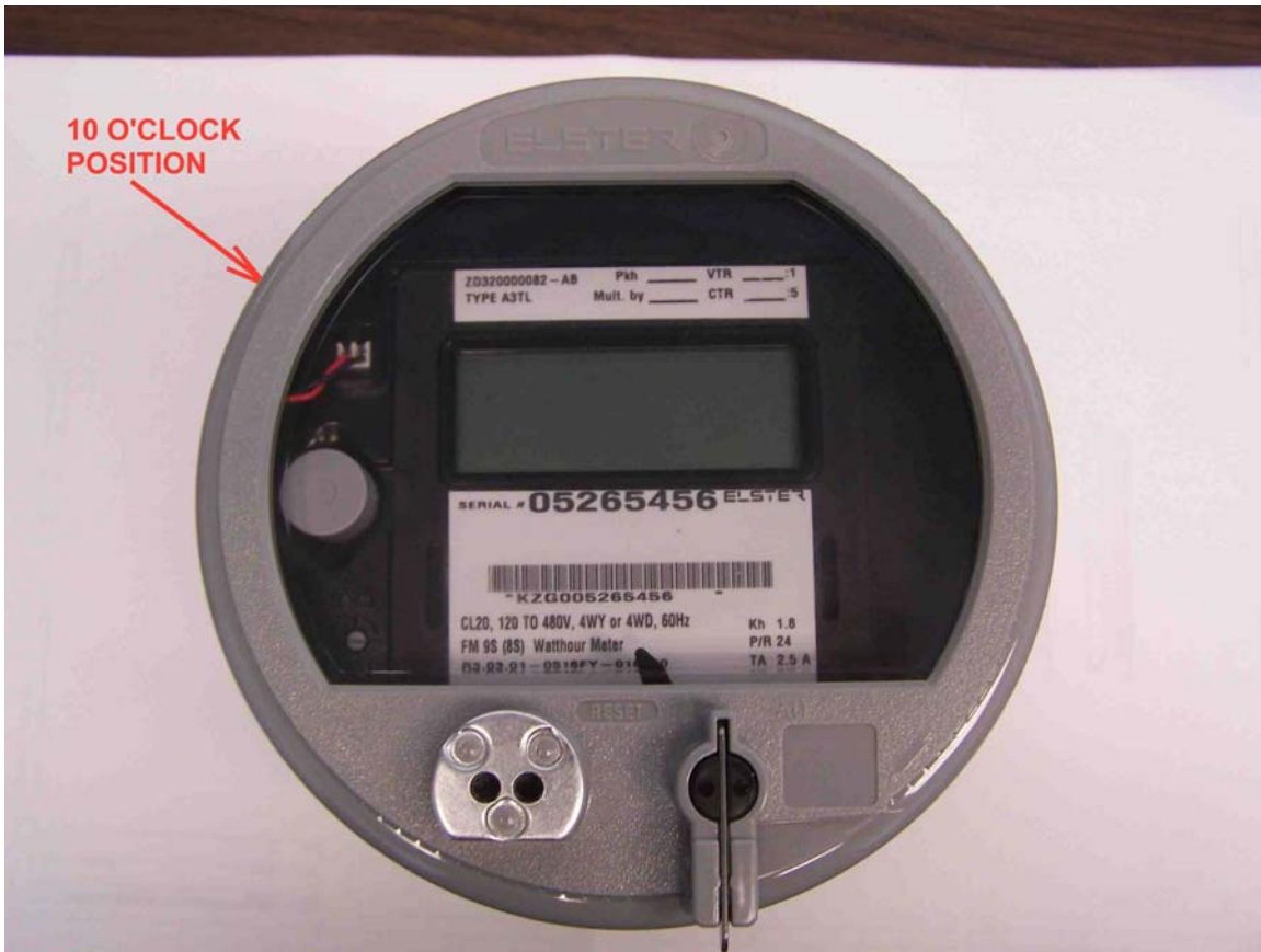
Photograph showing bar code position and 10:00 position for programming wand placement on meter.
