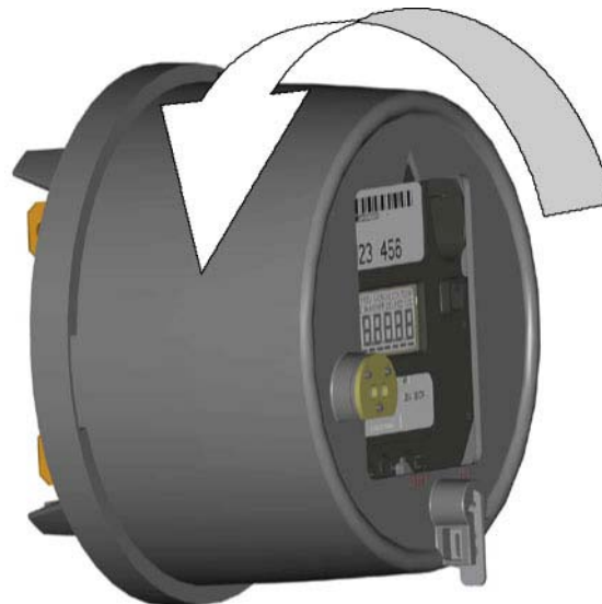
Figure 4-1: Removing the Meter Cover
