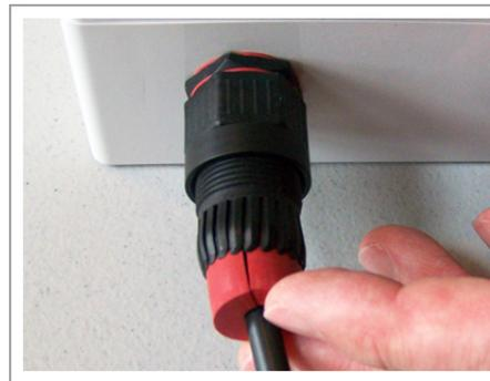
Figure 6.17. Slide cable bushing fully into connector B
