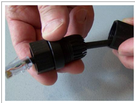
Figure 6.10. Thread cable through connector B
