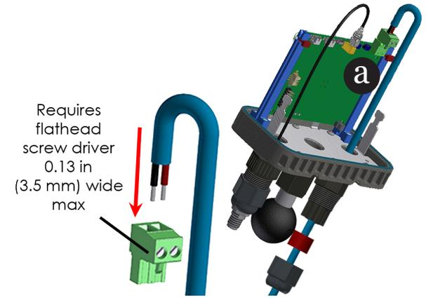
**Connect Stripped Wires to Green Terminal Block**
