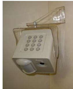
SafeScout mounted with u-shaped and corner brackets
