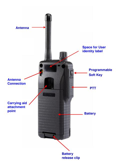
To ensure optimal performance from your terminal during half duplex calls (individual or group) please hold the unit vertically, with the half duplex microphone situated approximately 5cm away from the mouth.
