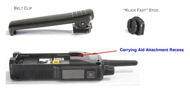
The Belt Clip and "Klick Fast" Stud are both attached at the carrying aid attachment recess on the rear of the terminal. When attaching or removing the belt clip or stud please fist remove the battery.
