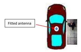
Should it not be possible to maintain the minimum safe distance between third parties and the radiating antenna, then action must be taken by the installer to reduce the potential for exposure at the specified minimum distance such that the Occupational Exposure limits are not exceeded.
