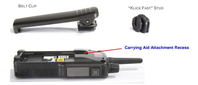
The Belt Clip and "Klick Fast" Stud are both attached at the carrying aid attachment recess on the rear of the radio. When attaching or removing the belt clip or stud please first remove the battery.
