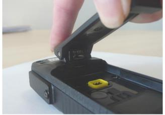
Use your thumb or thumb nail to compress the metal spring and release the belt clip. It is then possible to pull the belt clip so that it slides out of the carrying aid attachment recess.
