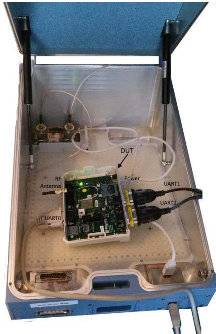
Figure A-1: Shield Box Cavity View
