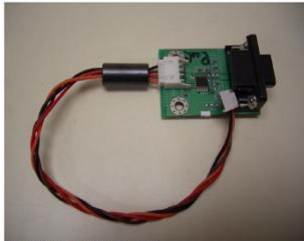
Platform debugging cable
