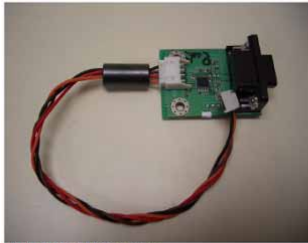
Platform debugging cable
