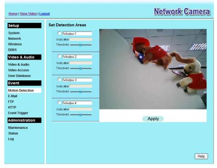
**Figure 27: Motion Detection**
