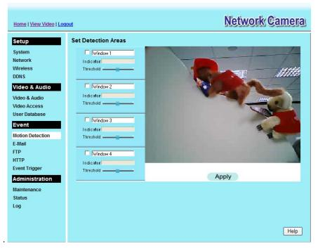
**Figure 36: Motion Detection Screen**
