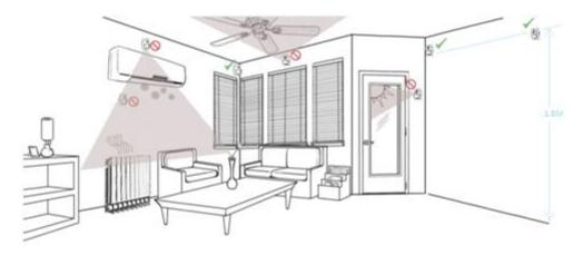
The recommended mounted position for a Motion Sensor should be 1.8M from the floor in the corner of a room. At this height, the device can detect a movement up to  $10M~(\pm 1M~)$  (see the following image). Also, in this position, the 90 degrees ( $\pm 10~degree$ ) fanshaped detection pattern can normally offer greater protection than mounting on a flat wall.
