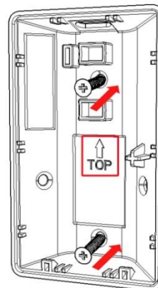
Flat Wall Installation
