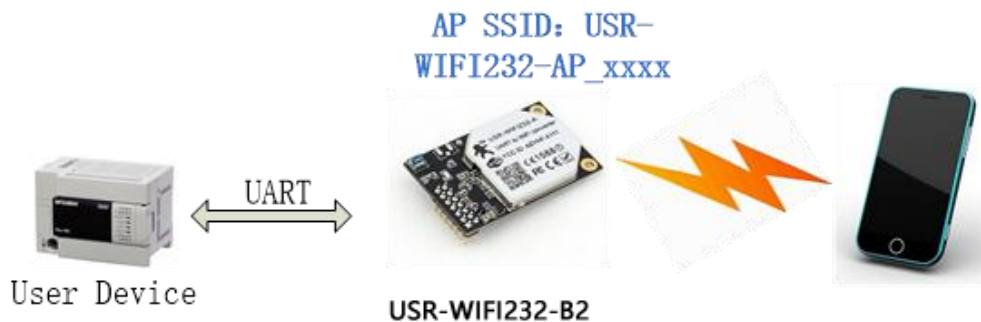
Figure 47 Wireless Control Application
