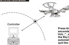
Press the 360°Flip button for 3 seconds until heard "tick. tick. tick.", enter auto-return mode, the Sky Hawkeye will fly backward automatically. Raise the joystick to quit the auto-return mode.
