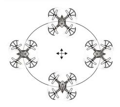
Press the Speed button for 3 seconds until heard "tick. tick. tick..", enter headless mode, the Sky Hawkeye will reset the direction. No matter what direction the head of Sky Hawkeye towards, it will fly back to controller when you pull back the direction joystick, it will fly forward when you push the joystick.
