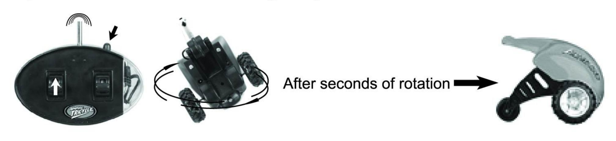
Make the tumbled vehicle return to standing up position (when the fore right wheel touch the ground)
