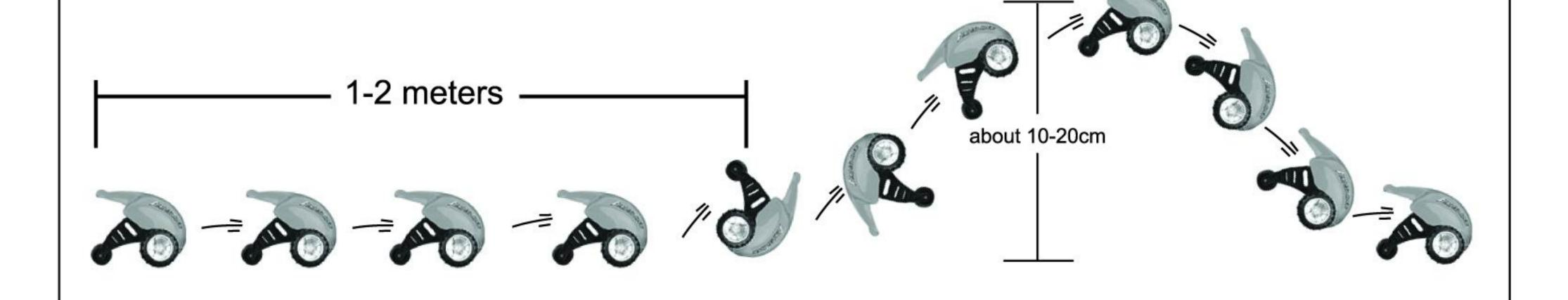
Make the tumbled vehicle return to standing up position (when the fore left wheel touch the ground).
