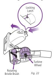
Blockages may cause your vacuum to overheat and shut down. To prevent this from happening, check potential blockage areas after heavy use or if you detect a loss of suction or poor cleaning performance.
