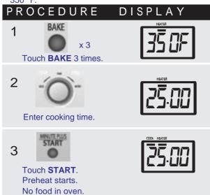
When the oven reaches the programmed temperature, a signal will sound 4 times.\*
