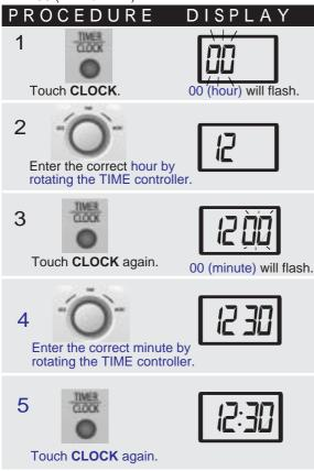
If the electrical power supply to your microwave oven should be interrupted, the display will intermittently show 88:88 after the power is reinstated. If this occurs during cooking, the program will be erased. The time of day will also be erased. Simply touch STOP/CLEAR and reset the clock for the correct time of day.
