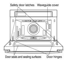
Check the oven for any damage, such as misaligned or bent door, damaged door seals and sealing surfaces, broken or loose door hinges and latches and dents inside the cavity or on the door. If there is any damage, do not operate the oven and contact your dealer or SHARP AUTHORIZED SERVICER.
