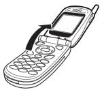
1. Active-flip: By closing this Active-flip, you can end a call. And the backlight will be automatically turned off.
