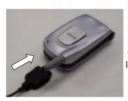
Use only the chargers approved by the manufacturer. Use of any unauthorized accessories may be dangerous and will invalidate the phone warranty if the accessories cause damage or a defect to the phone.
