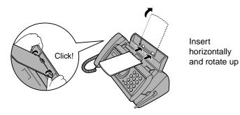
**Note:** The paper tray extension has a top side and a bottom side. If the tabs do not go into the holes, turn the support over.
