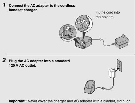
other material. Excessive heating may result and cause fire.
