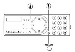
You can adjust the volume of the speaker, handset, and ringer using the up and down arrow keys.
