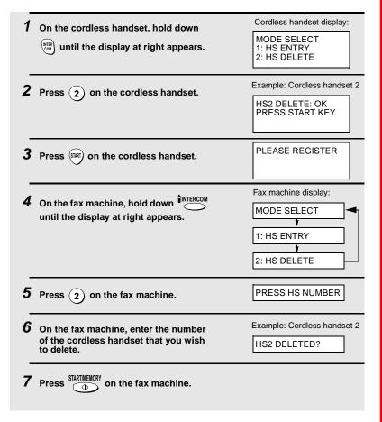
**Note:** To ensure correct operation, be sure to perform the deletion procedure both on the cordless handset and on the fax machine, as explained above.
