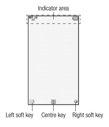
1. Till/ 🌋: Strength of received signal/Service out of range
