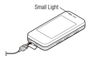
**2.** Connect the AC charger to an AC outlet.
