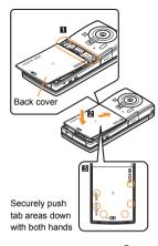
4 Slide the back cover lever in the direction of the arrow (<a>□</a>) to lock
