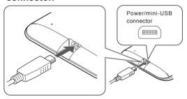
When charging starts, the battery indicator on the front side of the product (( ) turns red. When the product is fully charged, the battery indicator turns off.
