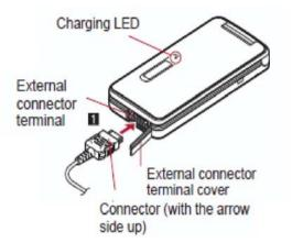
When inserting the AC adapter power plug into an outlet, charge alert is heard, charging LED illuminates, and charging starts
