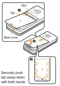
4 Slide the back cover lever in the direction of the arrow (4) to lock
