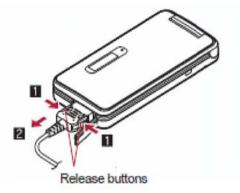
• Do not forcibly insert or remove. May cause damage to the external connector terminal and the connector or result in malfunction.
