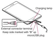
3 When you erect the AC adapter power plug and insert it into an outlet or insert the DC adapter power plug into a car cigarette lighter socket, the charging lamp illuminates and charging starts
