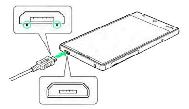
■ Insert Micro USB plug in correct orientation; otherwise, External Device Port may be damaged. Check contours and orientation of Micro USB plug, then insert it with tabs (O) facing down.
