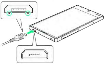
■ Insert Micro USB plug in correct orientation; otherwise, External Device Port may be damaged. Check contours and orientation of Micro USB plug, then insert it with tabs (O) facing down.
