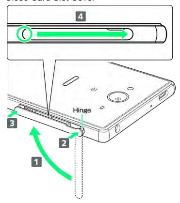
■ Lift Card Slot Cover in the direction of 1 and reinsert hinge as shown (2); place Card Slot Cover over the slot so that there is no gap between handset and Card Slot Cover, then push it in the direction of the arrow (3) to close.
