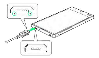
Insert Micro USB plug in correct orientation; otherwise, External Device Port may be damaged.
