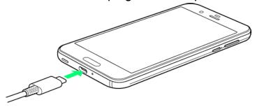
■ Insert Micro USB plug in correct orientation; otherwise, External Connection Jack may be damaged. Check contours and orientation of Micro USB plug, then insert it with tabs (O) facing down.
