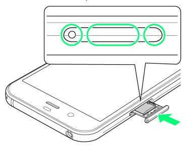
■ Push Card Slot Cap as shown (1 and 2) to close, then push it firmly all the way from circled area (O) to hinge as shown (3) so that there is no gap between handset and Card Slot Cap.
