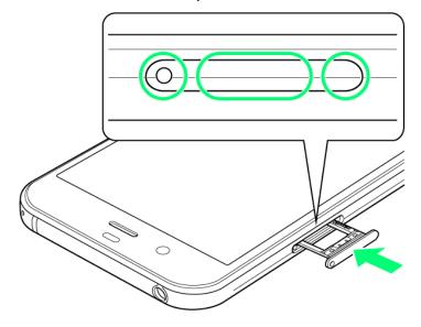
■ Push Card Clot Cap as shown (1 and 2) to close, then push it firmly all the way from circled area (O) to hinge as shown (3) so that there is no gap between handset and Card Slot Cap.
