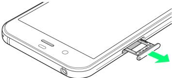
■ Do not pull USIM Tray forcefully or at an angle; damage may result. Gently pull it out horizontally by hooking a finger on it.
