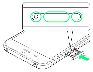
■ Push Card Clot Cap as shown (11 and 12) to close, then push it firmly all the way from circled area (O) to hinge as shown (13) so that there is no gap between handset and Card Slot Cap.
