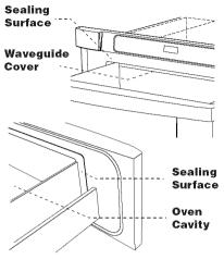
drawer, damaged drawer seals and sealing surfaces, broken or loose drawer guides and dents inside the cavity or on the front side of the drawer. If there is any damage, do not operate the Microwave Drawer and contact your dealer or a SHARP AUTHORIZED SERVICER.
