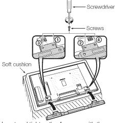
Insert and tighten the 4 screws with the screwdriver (supplied with the product) in the order of (1), (2), (3) and (4).
