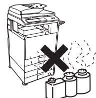
Installing the machine next to a diazo copy machine may cause dirty output.
