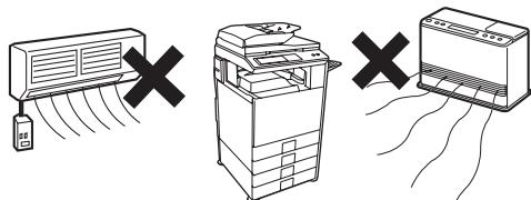
The paper will become damp and condensation may form inside the machine, causing misfeeds and dirty output.
