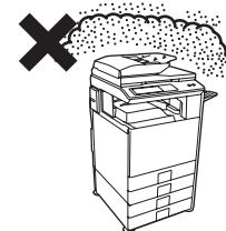
If dust enters the machine, dirty output and machine failure may result.
