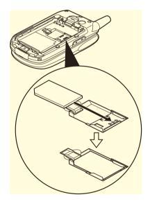
Position the battery with the printed side up. Insert its top end as illustrated into slot and insert the other end into position .
