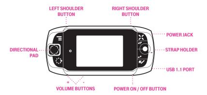
**DIRECTIONAL PAD (D-Pad)** Press up/down/left/right to scroll or move within text fields and navigate in games. The D-Pad "rocks" in four different directions and generally mirrors the behaviour of the trackball.
