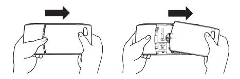
To replace the back cover, align the back cover with the body of the Sidekick and slide it into place. Take the reverse steps to remove the back cover.
