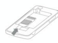
\*When changing the MicroSD memory card, first make sure that the phone has been turned off and then change out the card. If the MicroSD memory card is changed while the phone is still turned on, the data stored on the card may be destroyed or become unreadable.
