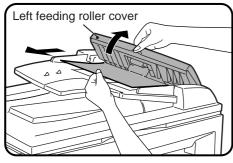
Open the left feeding roller cover and pull the original gently to the left and out from the document feeder tray. Close the left feeding roller cover.
