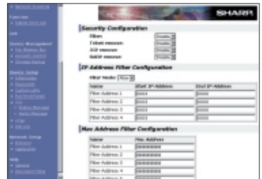
The IMAGER Home Page provides IP/MAC Address Filtering, so networked devices are restricted to authorized users only.
