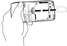
3 To remove the SIM card, use your finger to press down gently and slide the card right. When it's free of the slot, lift the card to remove it.
