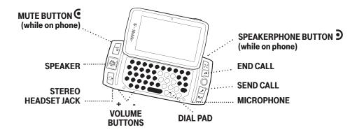
**SPEAKER** – When using the device as a handset, place the speaker, located in the D-Pad, to your ear.
