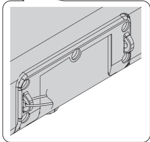
Loop the safety wires (not supplied) into each hole as shown and tie the safety wires to the LCD TV stand.
