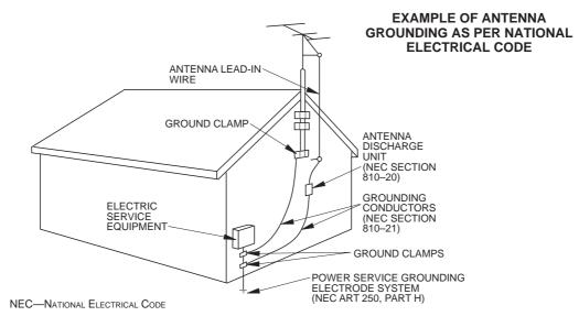
2. An outside antenna system should not be located in the vicinity of overhead power lines or other electric light or power circuits, or where it can come into contact with power lines or circuits. When installing an outside antenna system, extreme care should be taken to keep from coming into contact with power lines or circuits; contact with them might be fatal.
