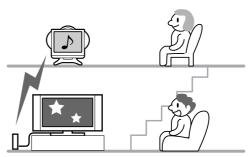
Even if the power supply of the Wireless Center is turned off, pictures and sound can be received by the main TV connected to the output terminals (through) and enjoyment is therefore possible even with a single television.
