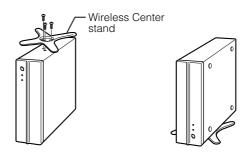
\* Failure to securely fasten the stand may cause the Wireless Center to tip over during use.
