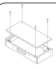
Start by removing the lid of the **Foot Box**. Remove the four Phillips head screws to free the lid, and it will pull straight up. Do not close the **Foot Box** until you have finished setting up and connected all of the cables.
