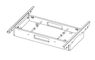
Use the four bolts and washers in the bag labeled <u>Foot Box Connect</u> <u>Hardware</u> to connect the **Foot Box** to the **Monitor Cabinet** and **Seat Cabinet** as shown to the left. Tighten the bolts with a 7/16" wrench. Note that this image does not show the **Monitor Cabinet** or **Seat Cabinet** so that you can easily see where the bolts attach. After thes bolts are tightened, tighten the outside bolts with an Allen wrench.
