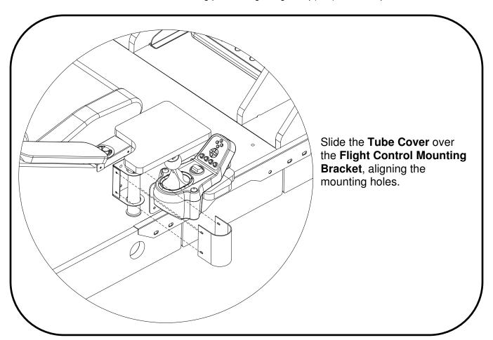
Using the four screws and washers you removed; attach the **Tube Cover** to the bracket you mounted. If your screwdriver is too long, you may need to remove the **Shifter** to tighten one two of the screws.
