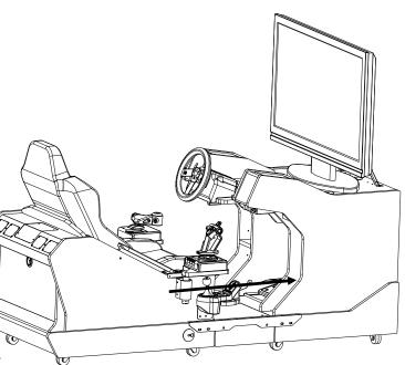
You can also install your computer in the rear cabinet. In order to do this, you will need some longer cables that are not included. Run the computer cables through the cabinet under the seat. These cables can be found at an electronics store or PI Manufacturing's website, www.PIMFG.com. The part numbers for these cables on PI Manufacturing's site are:
