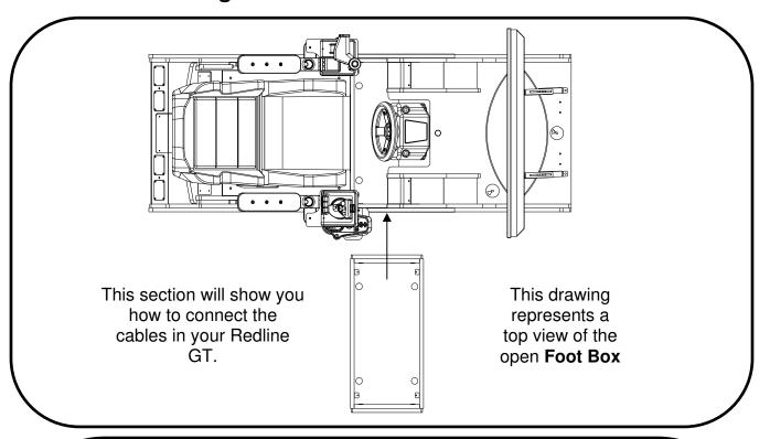
Connect the four sets of cables that you pulled into the **Foot Box** when you connected the cabinets. First, connect the cables with the 9-pin connectors, marked A. This cable powers the taillights and speakers in the **Seat Cabinet**.
