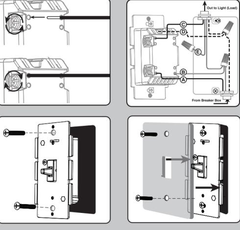
**Note:** The Traveler terminal is only used for 3-way or 4-way wiring and should remain insulated if the switch is being installed in a 2-way system (one switch & one load).
