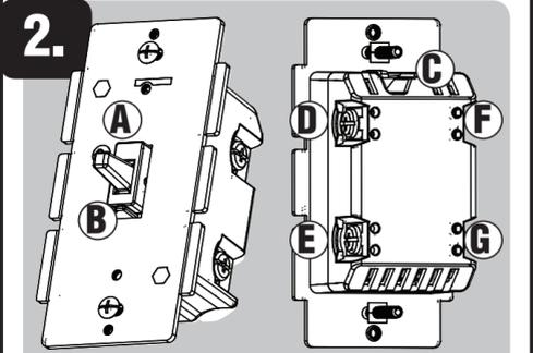
**A. UP** — (Press UP & release to turn Dimmer on, press up & hold increases brightness)
